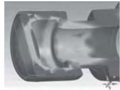
Simulation (FEM method) of the stress distribution under high pressure on housing and ceramic cap
