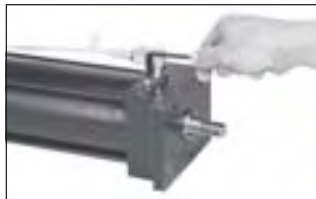
Bolt sensor to cylinder.
