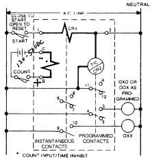
Standard Start — Close start switch to start, open to reset. (CX311 model count/inhibit input not at service voltage level). Unit resets on power failure.
