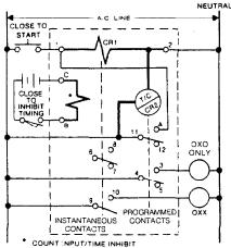
Momentary or Sustained Start - Close to time. Automatic reset at end of timing period with start switch open or closed. Note the jumper between A and 1 to provide "Lock In" power to the start circuit.
