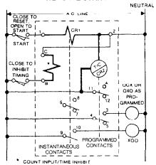
Reverse Start - Open switch to time; close to reset. Cycle progress is stopped without reset by closing inhibit switch. Unit does not reset on power failure. Battery retains cycle progress and setpoint.
