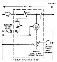
Standard Start — Close start switch to time; open to reset. Cycle progress is stopped without reset by closing inhibit switch. Unit resets on power failure. Setpoint is maintained by battery. Solid state delay contact actuates as interval (OXO) or delay (OOX) sequence as programmed by rocker switches.
