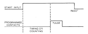
OO X PULSE AND REPEAT OPERATION — The contacts are energized at the end of the timing/counting cycle for a pulse which is user programmable. At the same time that the cycle is completed and the pulse output begins, the timing/counting cycle resets and begins again. This repeat operation continues as long as the start circuit is energized.
