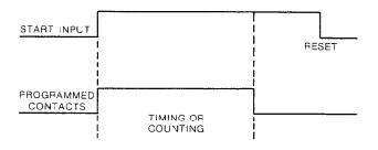
OOX PULSE OUTPUT OPERATION — The contacts are energized at the end of the timing/counting cycle for a pulse which is user programmable. See the Front Panel
