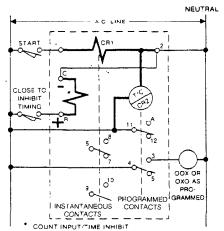
Standard Start - Close start switch to time; open to reset. Cycle progress is stopped without reset by closing inhibit switch. Unit resets on power failure. Setpoint is maintained by battery. Instantaneous contacts actuate with start switch. Programmed contacts actuate as programmed by rocker switches.
