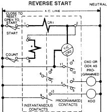
Reverse Start - Close start switch to reset, open to start. Unit does not reset on power failure. Battery retains cycle progress and setpoint.
