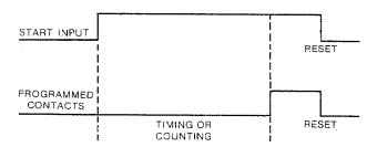
**OXO INTERVAL OPERATION** — The contacts are energized during the timing/counting cycle and then shut off at the end of the cycle.
