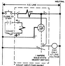
Momentary or Sustained Start — Close to start. Automatic reset at end of counting period with start switch open or closed. (Programmed for OXO output ONLY.) CX341 count/inhibit wiring snown. Note the jumper between 3 and 1 to provide "Lock in" power to the start circuit.
