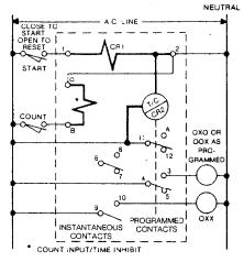
Standard Start - Close start switch to start, open to reset. Counts are registered when count switch opens. Unit resets on power failure. Setpoint is maintained.
