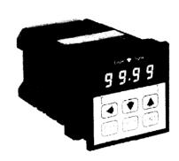
The SX110 is a microprocessor based control that combines a three-setpoint repeat cycle timer with an internal batch counter. The three setpoints on the repeat cycle timer function allows overlap or dwell between the two output timing intervals. The batch counter counts the number of repeat cycle operations that the timer performs, and automatically stops the timer operation after the user programmed number of cycles.
