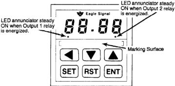
Pressing the SET key calls the prompted programming routine for the three setpoints. These are indicated with the "SEt1", "SEt2" and "SEt3" prompts. Each setpoint is displayed with the lease significant digit flashing. The position of the flashing digit can be changed using the key. The  $\triangle$  and  $\nabla$  keys increment and decrement the value of the flashing digit. The ENT key enters any setpoint changes into memory.
