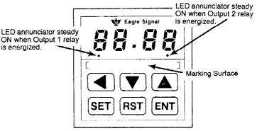
Pressing the SET key calls the prompted programming routine for the three setpoints. These are indicated with "SEt1" and "SEt2" and "rEPt" prompts. Each setpoint is displayed with the least significant digit flashing. The position of the flashing digit can be changed using the ◀ key. The ▲ and ▼ keys increment and decrement the value of the flashing digit. The ENT key enters any setpoint changes into memory.
