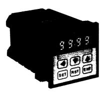
The SX410 and the SX430 are dual setpoint timers featuring an inhibit function that allows the timing operation of the units to be stopped without resetting the timed value or the outputs.
