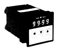
The SX460 is a dual output timer with two independently programmable, timing interval setpoints. The two outputs can be programmed to operate either simultaneously or in sequence, providing the equivalent operation of two interval timers. The sequential output operation can also be used to provide repeat cycle timer operation.
