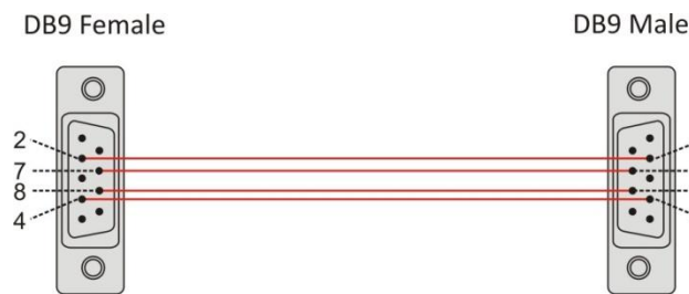
Figure 27 – Building an extension cable
