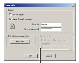
The "Return call" function is only available for specific device types with an active modem connection. Here you must enter the number of the PC that will be called by the device.
